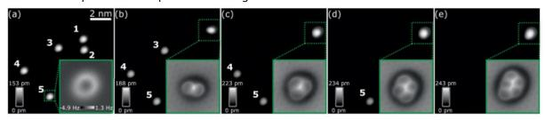
Our home built machine is currently optimized for investigating individual atoms and small clusters which are placed and altered on a Cu(111) surface (above figure shows the atom by atom assembly of a cluster consisting of five iron atoms; the insets are acquired in the AFM channel, while the overview images were recorded in STM mode) [2,3]. We employ CO terminated tips, which allow us to artificially create small clusters atom by atom and image the created structures with atomic resolution [3].
